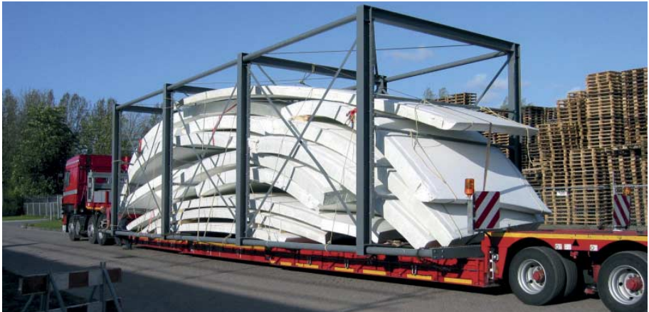
FIG. 82 Open container at Holland Composites with the roof segments ready for shipment
