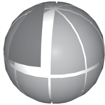
FIG. 65 Schematic drawing of the proposed division: 2 x 8 spherical segments in GRP
