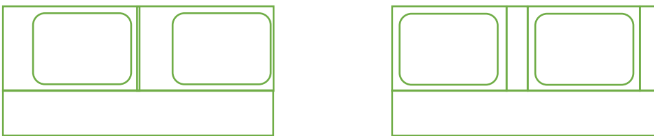
Figure 12: Panel configurations that )combine SGMm and ICMm/ICRm layout (left) and minimize window frame area (right)
