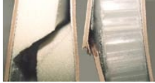
Figure 11: Foam core (left) and honeycomb (right). Retrieved from Carbon-core (Carbon-Core Corporation, 2020)
