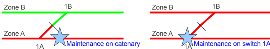
Figure 5.2: Illustration of the effect of coupled switches on TVPs
