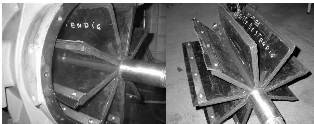
Figure 7.4: Thermally insulated sluice rotors.
