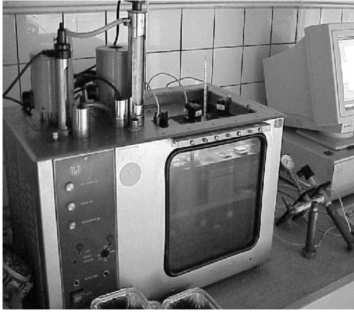
Figure 4.4: Equilibrium vapour pressures above moist fines were determined using cylindrical containers. These cylinders were filled with cake, pulled vacuum, and immersed in a hot oil bath.
