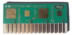
(a) 5 LFPAK56 packaged devices on a PCB.
