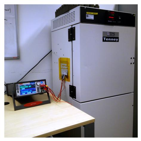
Figure 5.16: Calibration measurement setup, a Keithly 2450 SourceMeter is used to measure the Vf with the device in the TPS thermal chamber at a know stable temperature.
