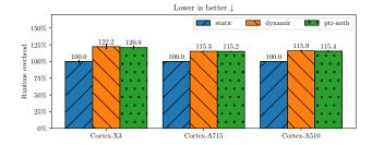
**Figure 15.** Overheads of pointer authentication.
