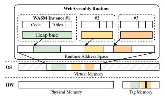
**(b)** External memory safety enforced by MTE. The linear memory of each instance is assigned a unique tag, which is stored in the heap base pointer and is used for effective address calculation.
