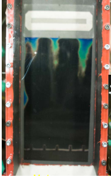
Figure 6.1: Picture of the test section sample B2_P1_2mm, blowing ratio M=1
