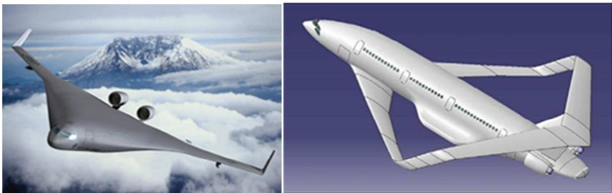
**Fig. 1.1: Examples of advanced non conventional aircraft configurations for the future: the blended wing body (left) and the joint-wing aircraft (right), also known as Prandtl-Plane (Frediani, 2004).**
