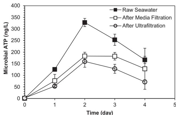
**Fig. 10.** Monitored bacterial growth potential based on microbial ATP using the ATP-filtration method. Samples were collected from raw seawater (■), after media filtration (□) and after ultrafiltration (○) of a pilot-scale plant (the Netherlands). Data of Day 0 is the initial microbial ATP concentration after inoculation.
