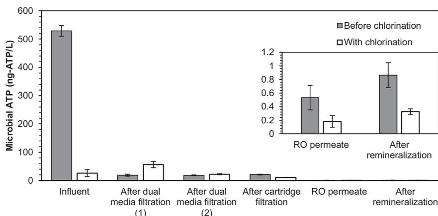
**Fig. 8.** Microbial ATP concentrations measured using the ATP-filtration method for samples collected through the treatment processes of a full-scale SWRO desalination plant. All data are plotted as average ± standard deviation (n = 3).
