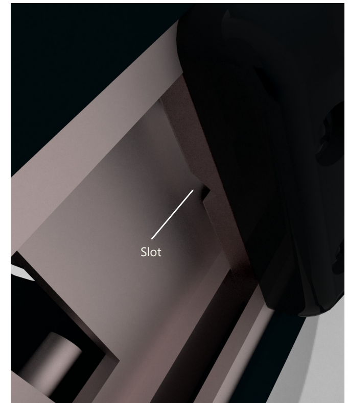
figure 60 : When the rod rotates it free's up a slot in the part connected to the tablet arm. Note, the vertical adjustment rod is not shown in this figure.
