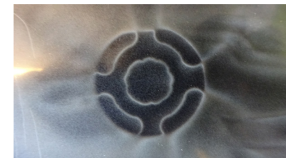
figure 53 The magnetic field boundaries of the portrait landscape mode magnet.
