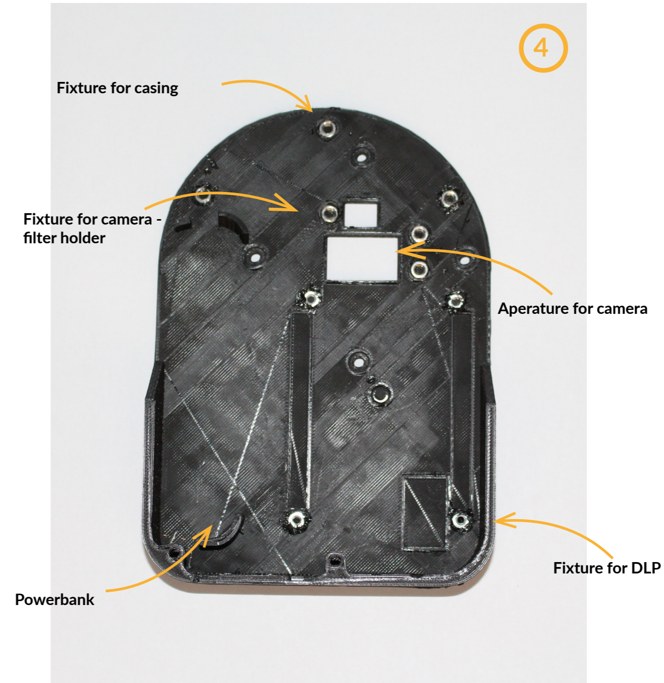
Figure 29, Assembly of baseplate
