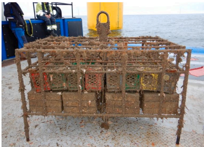
Fig. 4. Picture taken on board after the retrieval of an on-scour cage after it had been submerged for approximately 9 months.
