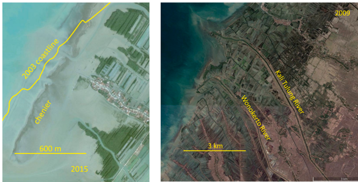
Fig. 26. Example of chenier formation Demak, Indonesia (Google Earth image) by (a) self-organization of eroded coastal sediment and (b) riverine sand input.
