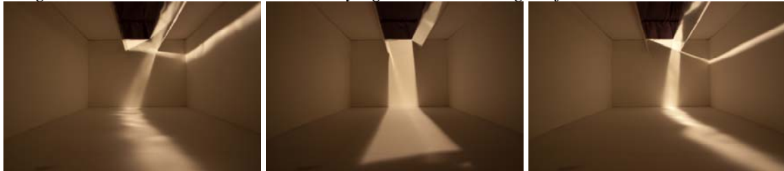
Longitudinal cut – 2.5 cm thickness – varying inclination – high reflective material
