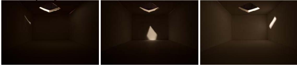
Diamond opening – 2.5 cm thickness – inclined south - translucent material
