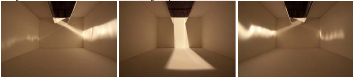
Longitudinal cut – 2.5 cm thickness – high reflective material
