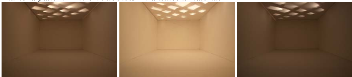
Diamond pattern – 1.0 cm thickness – translucent material
