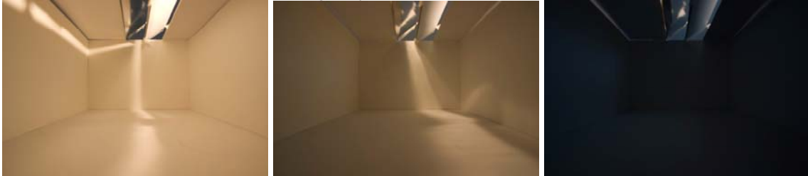
Opening east - double reflection – high reflective material
