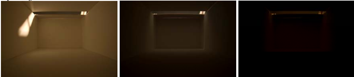
Opening north – double reflection – high reflective material
