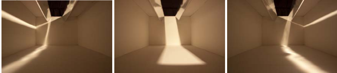
Longitudinal cut – 2.5 cm thickness – outward inclination – high reflective material
