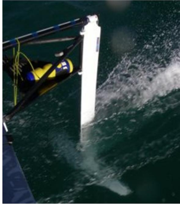
(a) Daggerboard and lifting hydrofoil ('T-foil'), showing trailing edge flap that is controlled by bow mounted wand sensor.
