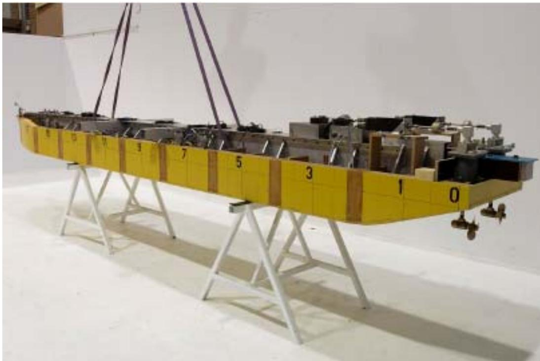
Figure 3 The segmented ACS vessel for the project PELS-I
