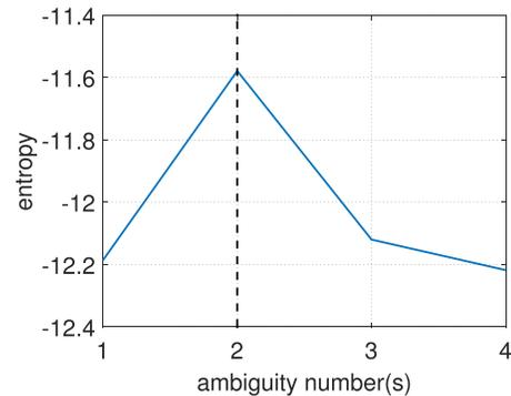
Fig. 14. Entropy of the inverse Radon image. The true ambiguity number is indicated by the black dash vertical line.
