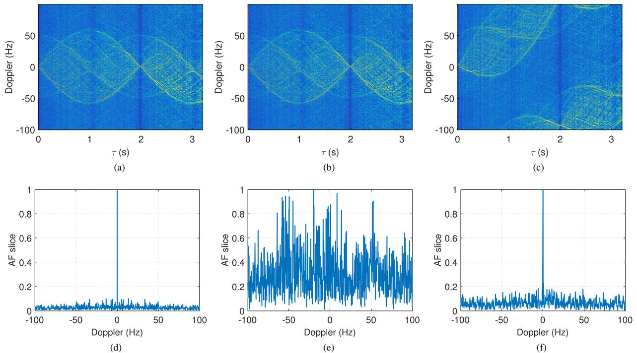
Fig. 5. AF of the radar echo. (a) MM case. (b) MMLT case. (c) MMQT case. (d) Slice of the MM case at  $\tau = 0$  s. (e) Slice of the MM case at  $\tau = 1$  s. (f) Slice of the MM case at  $\tau = 2$  s.
