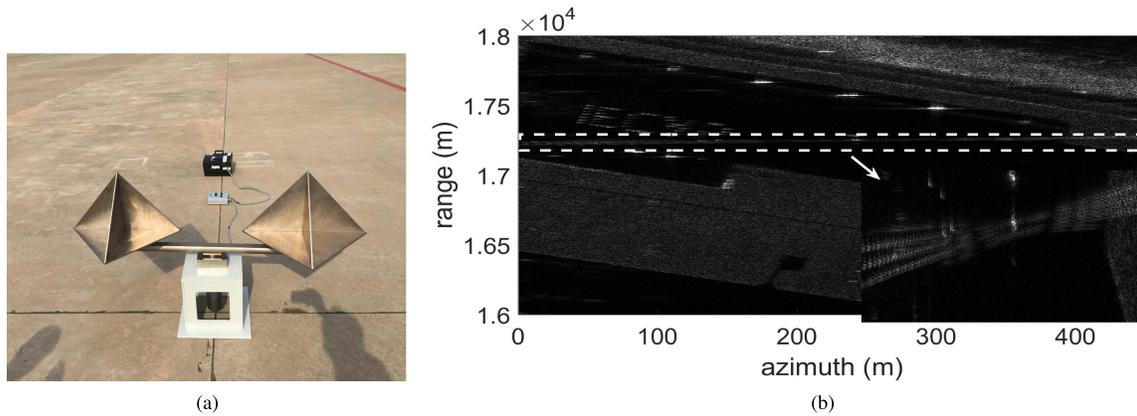
Fig. 10. Rotating corner reflectors located in the airport. (a) Rotating corner reflectors. (b) SAR image of the interesting area.
