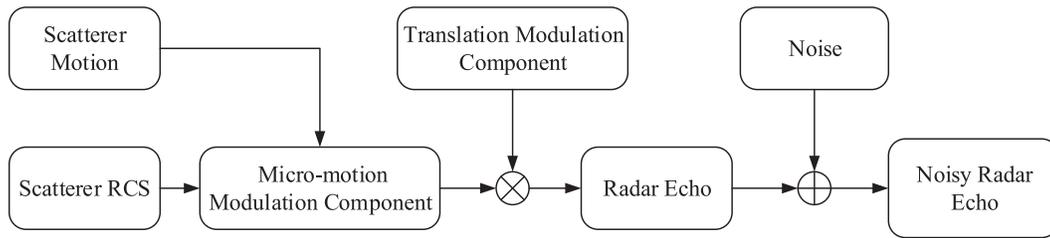
Fig. 3. Flowchart of the coning motion simulation.
