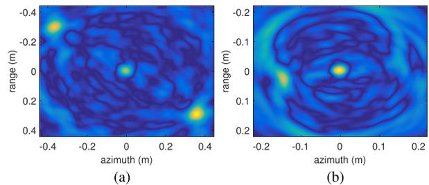
Fig. 15. Inverse Radon image with different ambiguity number. (a) Ambiguity number is 2. (b) Ambiguity number is 1.
