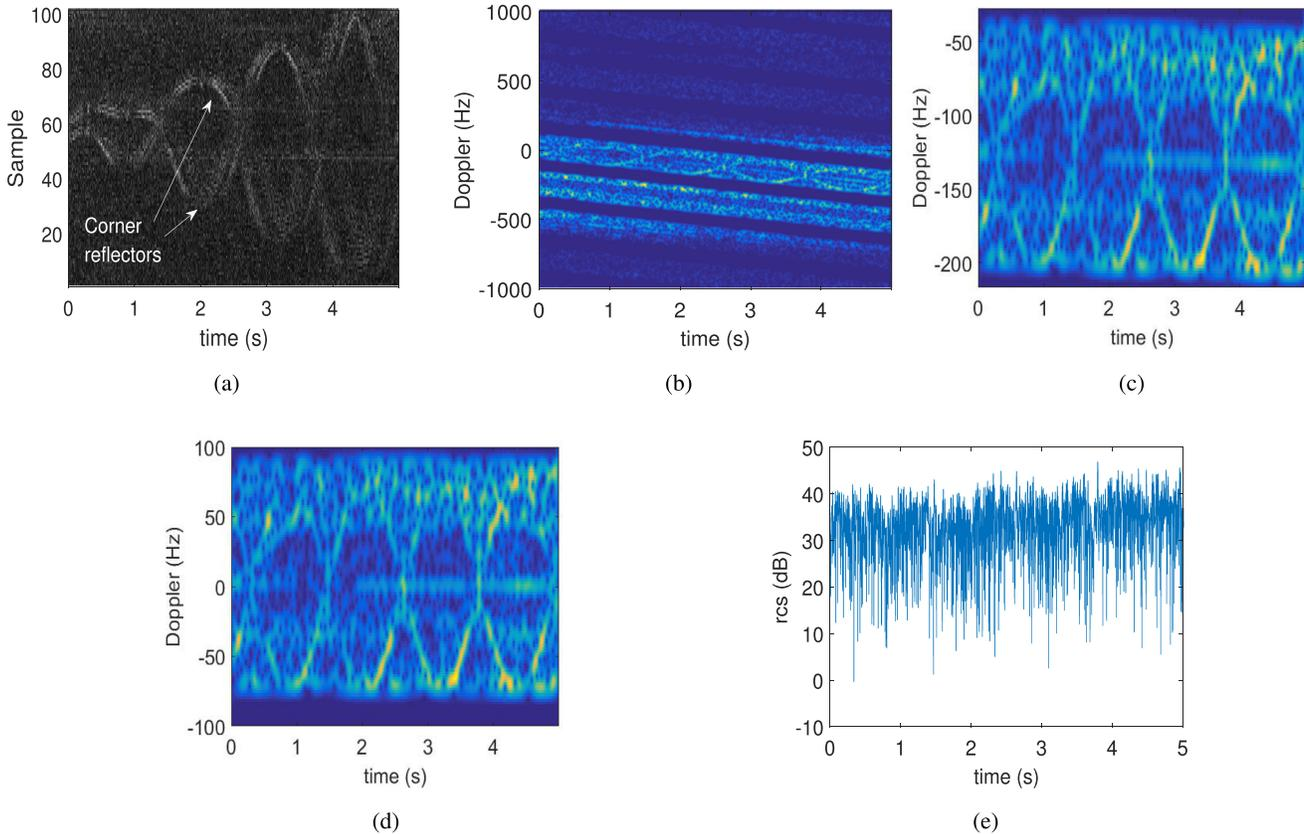
Fig. 12. (a) Range-compressed and azimuth-uncompressed signal. (b) STFT of the azimuth signal. (c) STFT of the preliminary compensated and filtered azimuth signal. (d) STFT of the m-D signal. (e) Uncalibrated RCS of the target.
