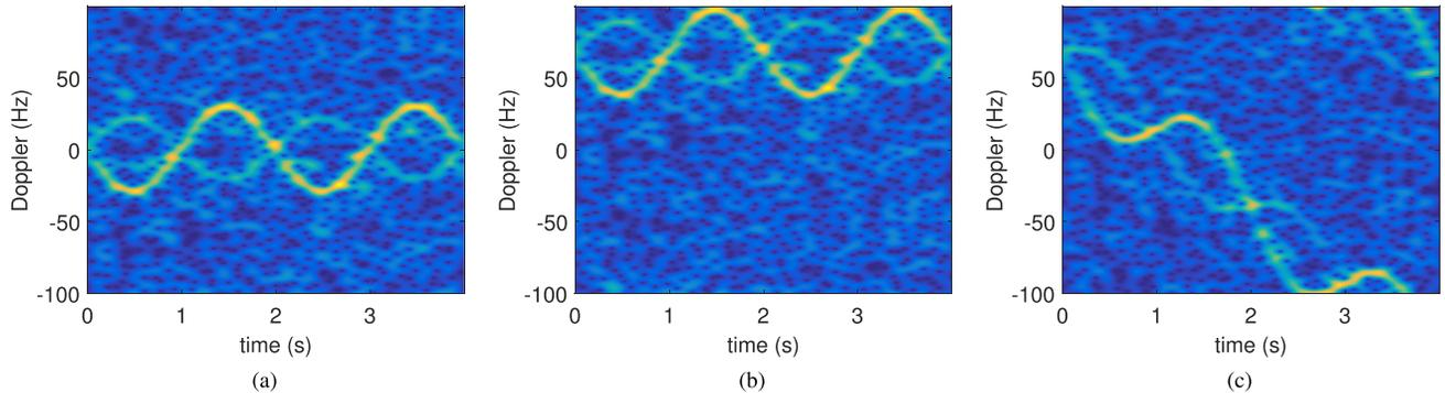
Fig. 4. STFT of the radar echo. (a) MM case. (b) MMLT case. (c) MMQT case.
