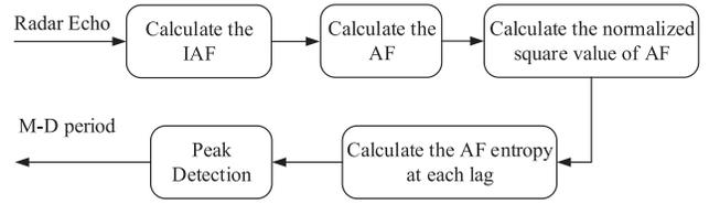
Fig. 1. Flowchart of AF entropy-based m-D period estimation.
