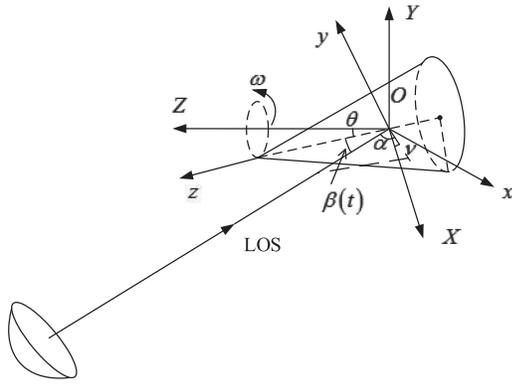
Fig. 2. Cone target model.
