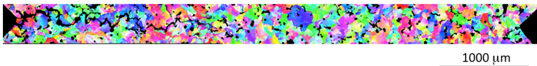
Figure 7.9 Large scale EBSD measurement through the entire thickness, the size of this scan is 6000 \times 700 \mu\text{m}^2 . Color coding is according to inverse pole figure legend of Figure 7.4.
