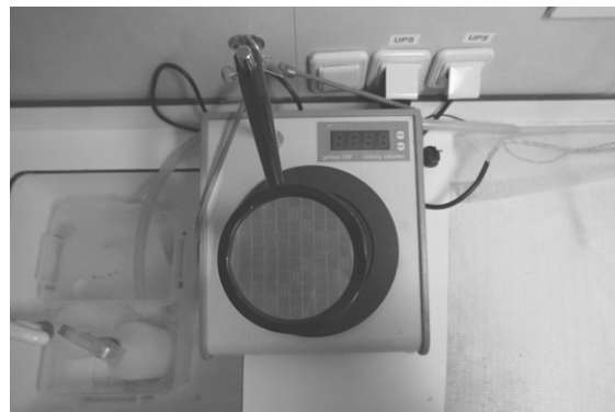
Galaxy 230 colony counter, used for bacteria/coliform. In collaboration with TUBITAK research Institute Wientjes, C. (November 2022)
