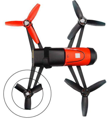
Fig. 6: Reduced rotor diameter by [4 cm] on right-aft rotor
