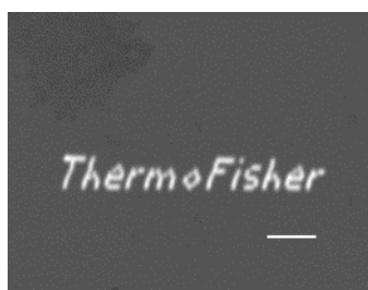
Figure 4.24: BSE image of the Thermo Fisher logo deposited using FEBID in the Phenom XL G2 system. The scale bar is 100 μm.
