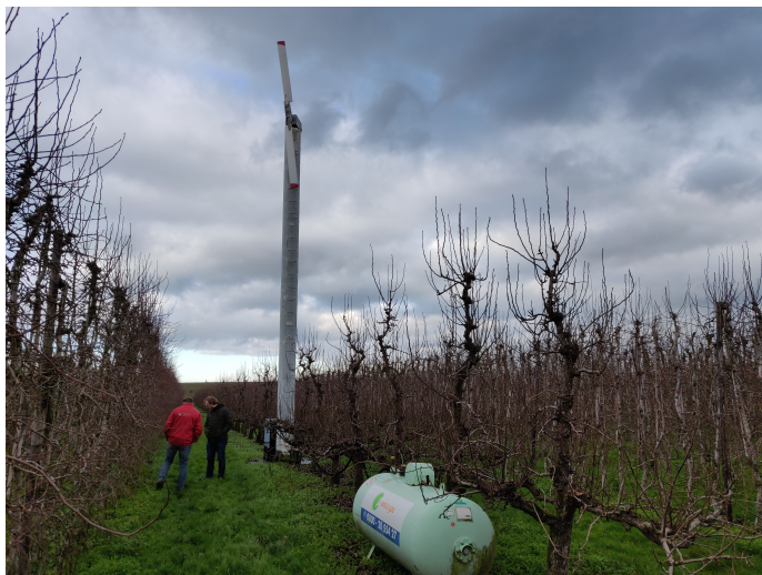
Figure 2: The wind machine in the pear orchard, with the engine mounted at the bottom of the tower. In the back, the dike is visible.
