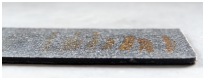
Figure 34. The hot press CB2 sample, including the dyne solution by Arends Corona Treatments.
