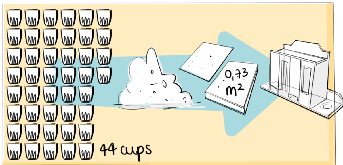
Figure 79. Upcycling: 44 cups of coffee, to SCG, to 0.73 m 2 panel, to a 7-compartment Kovivol.
