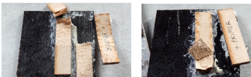
Figure 37. CB2 sample adherence test with and without primer: hot press sample (left) and oven sample (right).
