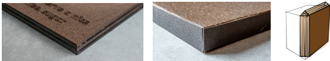
Figure 74. The sides of the laser cut condiment organizer (left), with an edge band edge (middle) and CNC-milled (right).
