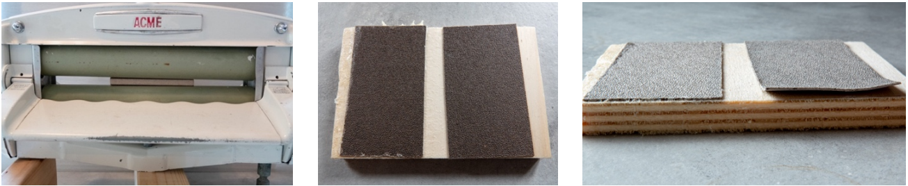
Figure 39. Adhesion press set-up (left), plywood with CB1 laminate adhered by BiolImpact (middle, left side) and wood glue (middle, right side), results after dishwasher test (right).
