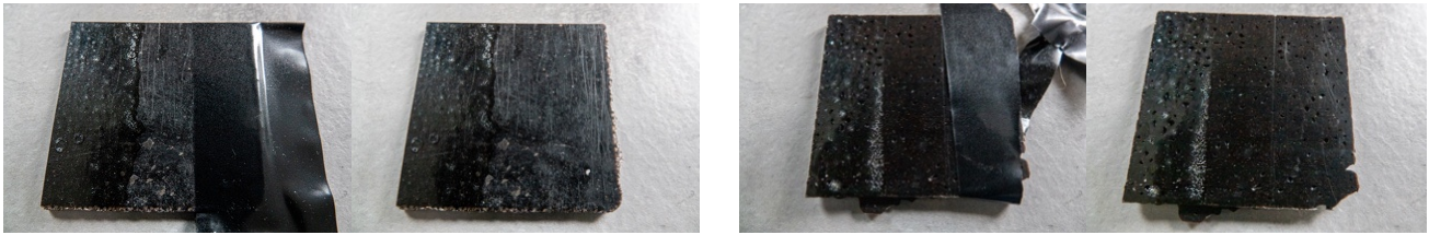
Figure 36. CB2 sample UV test before and after: hot press sample (left) and oven sample (right).
