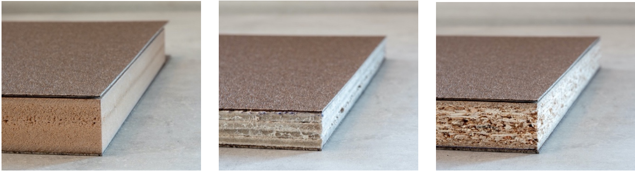
Figure 40. Side view of potential panel combinations, with Resysta NoWood (left), ECOR (middle) and EcoBoard (right).
