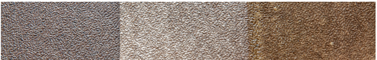
Figure 27. CB1 laminate dishwasher test: before (left) and after without (middle) and with coating (right).
