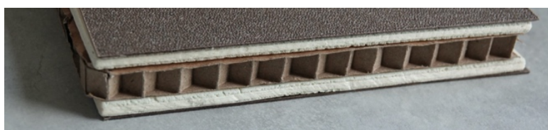
Figure 82. Example of multilayered core, including two sheets of triplex wrapping a cardboard honeycomb layer.
