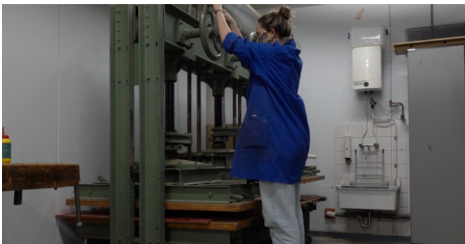
Figure 71. Laminating other side of the panel by sheet press.
