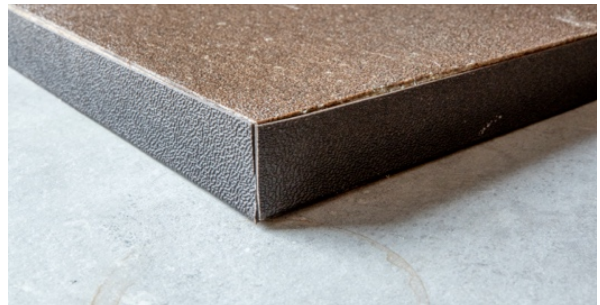
Figure 48. Scrap material of the CB1 laminate, draped around an old filament coil (left) and used to cover the proposed optimized panel (right).
