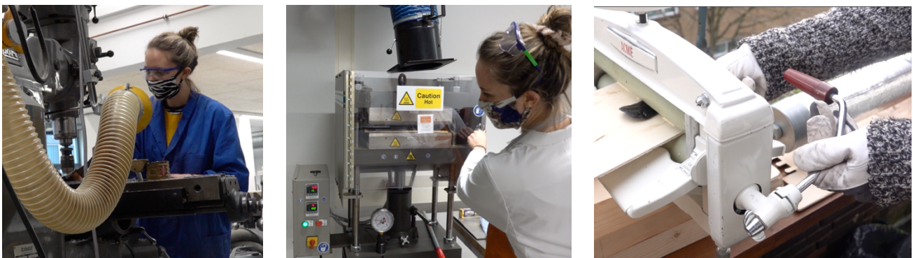
Figure 83. Pictures of me milling in PMB, hot pressing at Applied Labs and extruding at home.
