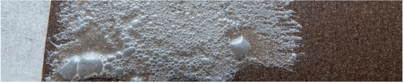
Figure 38. BiolImpact adhesive when sprayed onto the CB1 laminate.
