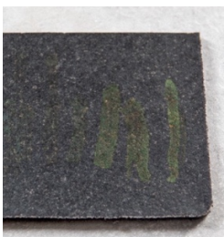
Figure 34. The hot press CB2 sample, including the dyne solution by Arends Corona Treatments.
