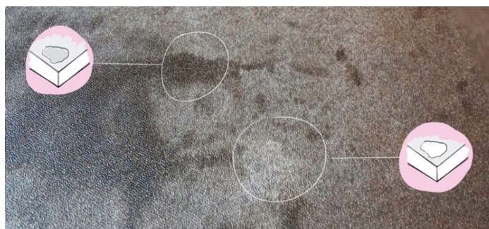
Figure 11. CB1 laminate discoloration caused by coffee corner use in the displayed situation in figure 10 for 39 days.
