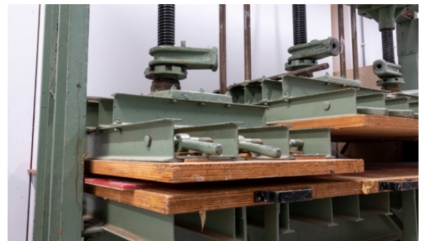
Figure 71. Laminating other side of the panel by sheet press.
