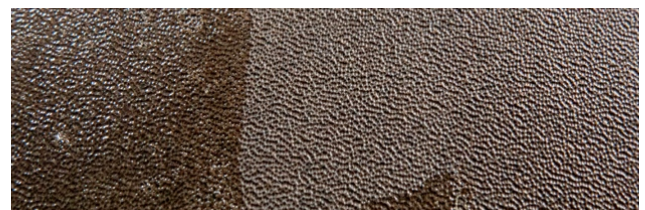
Figure 29. CB1 laminate UV test before and after: with (left) and without coating (middle) and covered (right).
