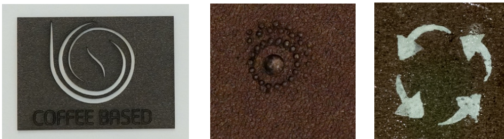
Figure 51. CB1 communication test results by laser cutting (left), stamping (middle) and painting (right).
