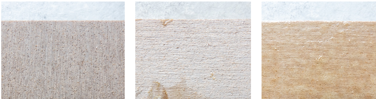
Figure 42. Resysta NoWood dishwasher test: before (left) and after without (middle) and with coating (right).
