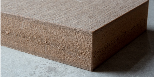
Figure 41: The chosen core: Resysta NoWood by FiberPlast.
