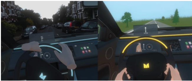
Figure 3. Images of VRHEAD in the first (left) and last (right) iteration. In the first iteration, the environment consisted of a static 360-degree photograph, while in the last iteration it is an abstract looping animation.
