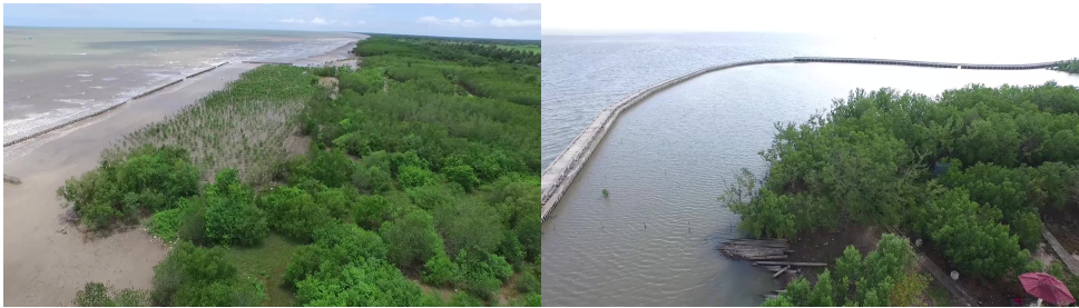
Figure 1.2: Examples of mangrove restoration project including soft solutions (left panel) and hard solution (right panel) along the Mekong Delta coast, Vietnam.
