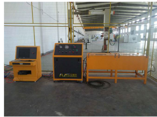
Fig. 12. Short-term burst pressure test system.
