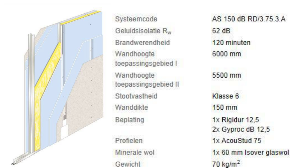
figure 5.9 partition walls (left) technical specification (right)
