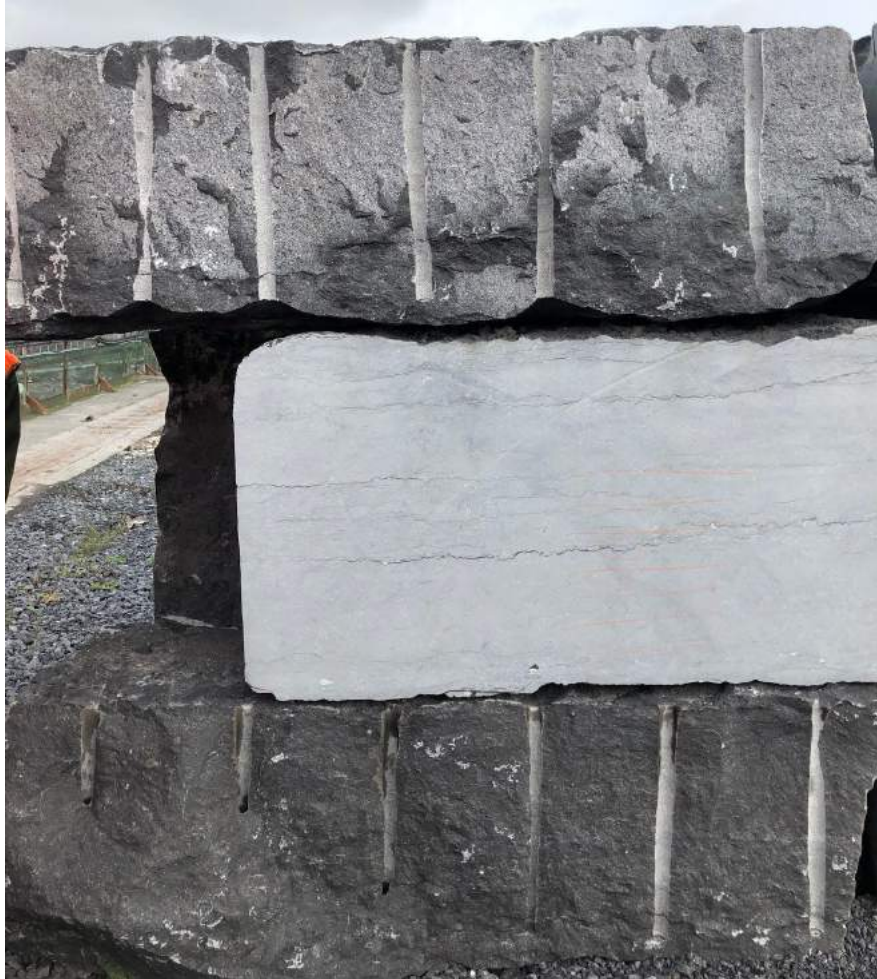
Fig. 6 | Carrières du Hainaut, Soignies, Belgium; holes visible in a limestone surface after the pneumatic drill.
