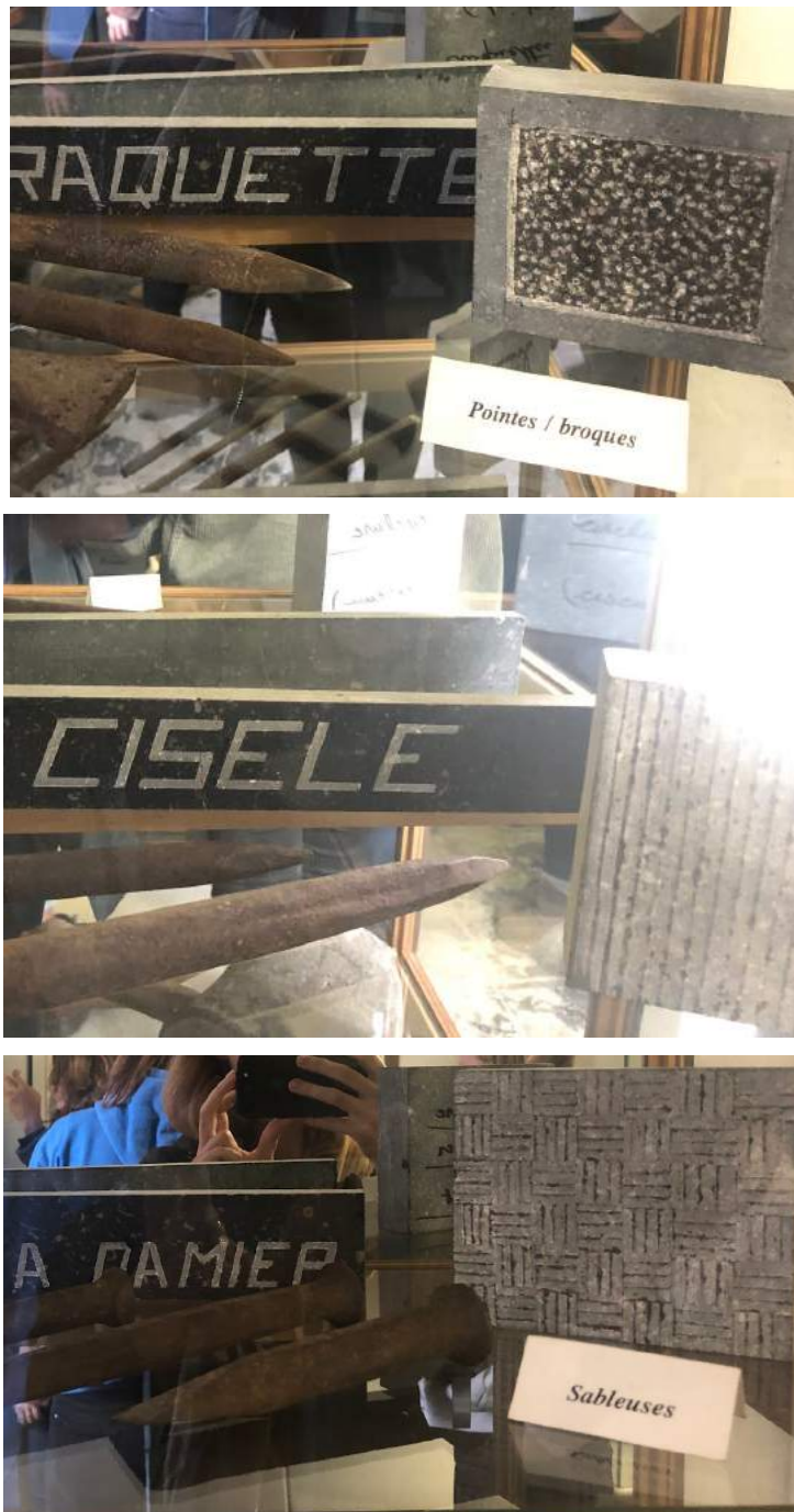
Fig. 9 | Photographs of different processed surface of limestone and the tools, which were used. Photographs have been taken in the Documentation Centre of Blue Limestone in Soignies ( Le Centre de Documentation de la Pierre Bleue Durée).
