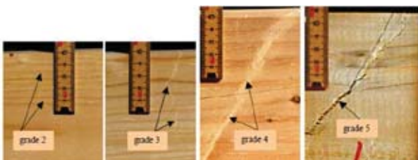
Figure 1: Classification of CF's grades in softwood [9]
