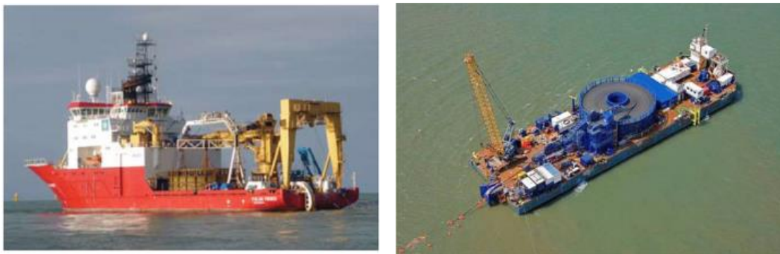
Figure 2.7: Left: Cable laying vessel, Right: Cable laying barge
