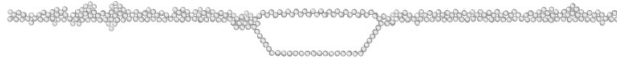
Figure 6.16: Contact with nano-scale asperities for case AB. Atoms that do not belong to the interface, i.e. that have FCC structure type, are excluded.
