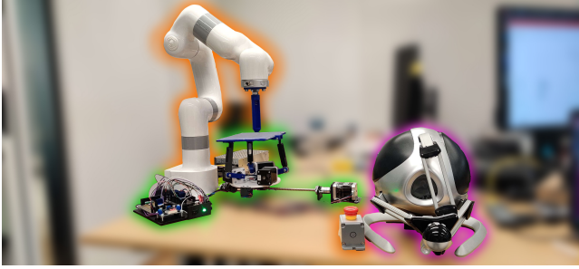
Figure 5: The experimental setup. The robot (Ufactory lite 6) is highlighted in orange with an extension that holds a whiteboard marker, power supply, and emergency button. Highlighted in green is the steward platform attached to a lead screw contraption and the motor drivers. Highlighted in pink is the haptic device (Novint Falcon).
