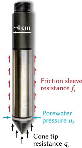
Figure 1.3: An example of a cone penetrometer (CPT) and the measurements it collects.
