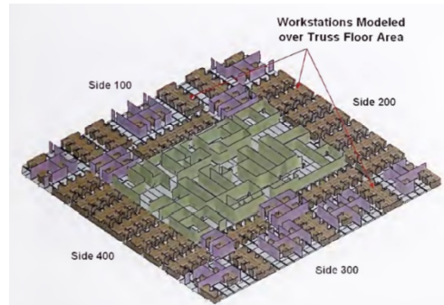
Fig.29 Model of the 96 th floor of WTC 1, including interior. (NIST, 2005).
