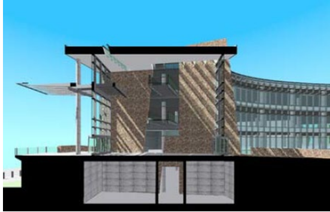
Fig.34 Section of the lobby showing a blast-resistant wall between the lobby and the office space (Pollalis, 2006).
