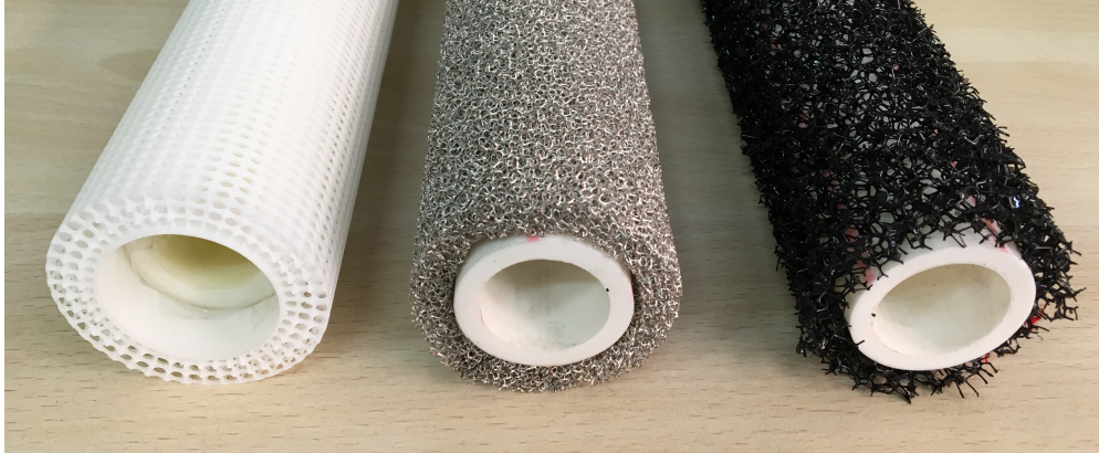
Fig. 1 Examples of porous coated cylinder types, illustrating the differences in porous coating structures that are used to treat cylinders as a form of passive noise control (from left to right: SPCC, MFPPC and PPCC).
