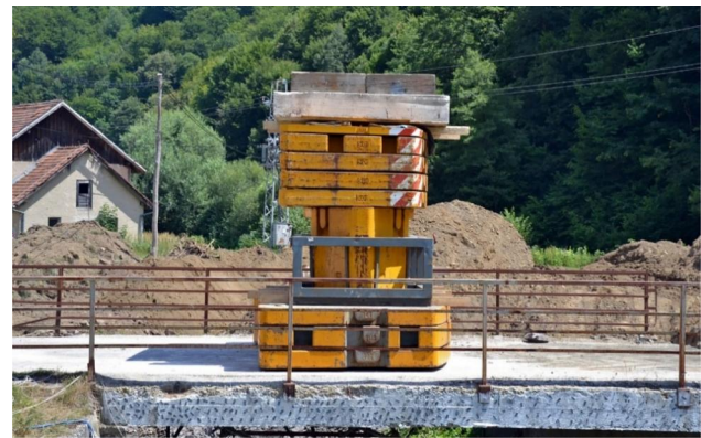
Figure 12. A proof-load test following a SLT on a test bridge in Slovenia.
