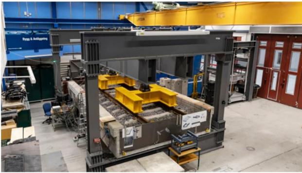
Figure 18. View of the full-scale trough bridge tested at the LTU lab.
