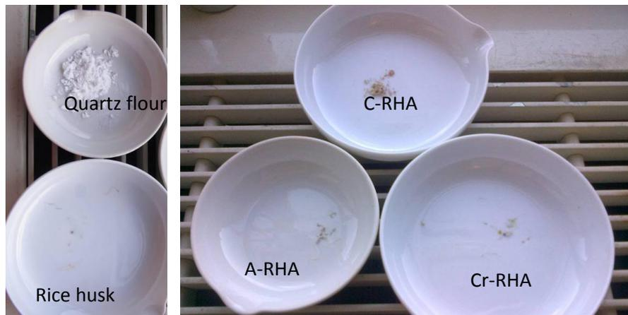
**Figure 20. Residues after ignition in the experiment of non reactive silica content**
