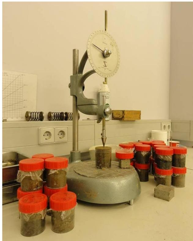
**Figure 28. Fall cone test for undrained shear strength identification**
