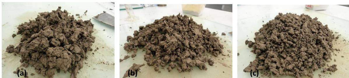
Figure 25. Clay after mixing with lime and RHA (lime : A-RHA = 1).
