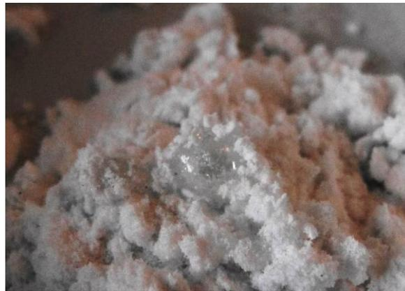
Figure 23. Partly quartz transferred to another form of crystal after ignition at 950°C
