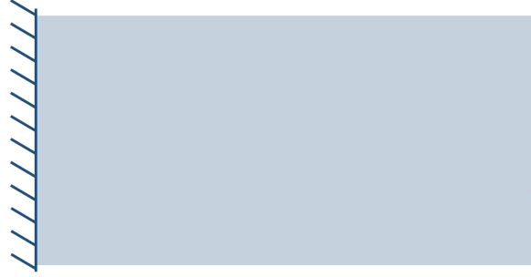
Figure 6.1: The design requirements for the cantilever beam. A load is applied on the middle of the right edge and the left side is fully clamped. The aspect ratio of the design space is 2:1 and 80x40 elements are used to discretize the structural analysis.
