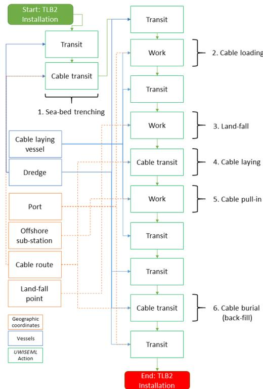
Figure 3.4: Installation process flow for the TLB (Trench Lay Burial) installation method.
