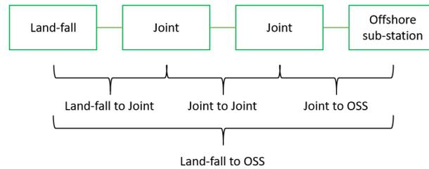
Figure 3.5: Classification of the different types of power cables used for an MIP.
