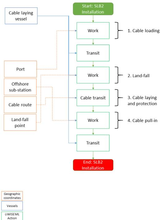
Figure 3.3: Installation process flow for the SLB (Simultaneous Lay Burial) installation method.
