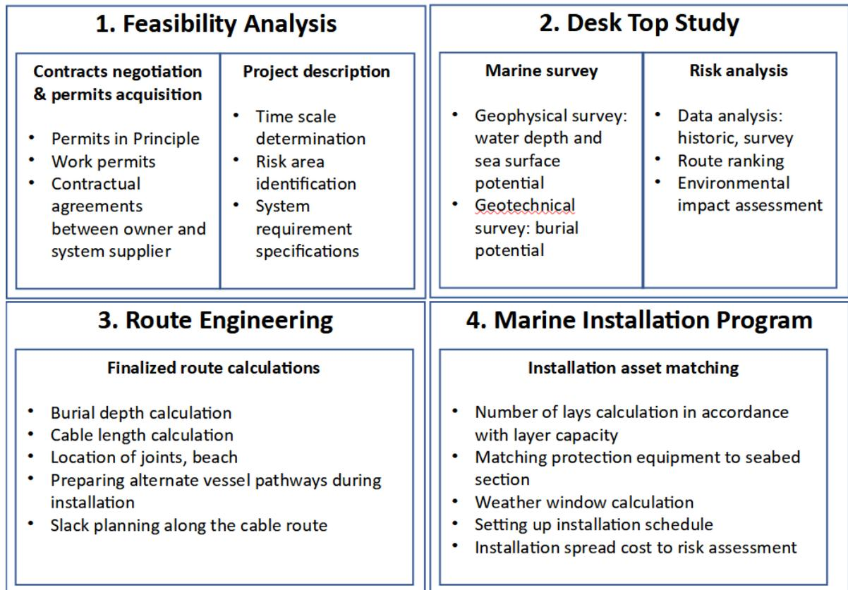
Figure 2.1: The four stages of a cable installation plan listed in order with their key objectives [9].
