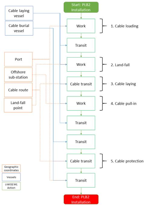
Figure 3.2: Installation process flow for the PLB (Post Lay Burial) installation method.
