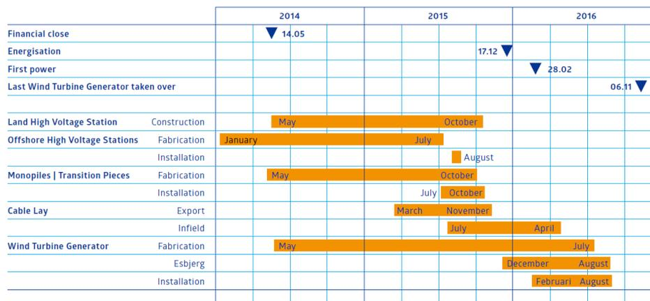
Figure 5.1: Gantt chart depicting the time consumed for the installation activities of the Gemini offshore wind farm. [24]
