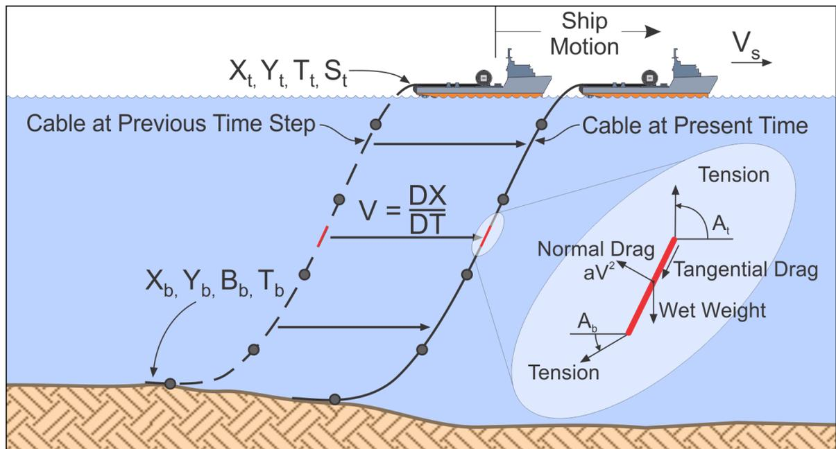
Figure 3.1: Representation of the dynamic forces experienced by a cable during the lay process captured on high fidelity mathematical models such as Makailay [14]
