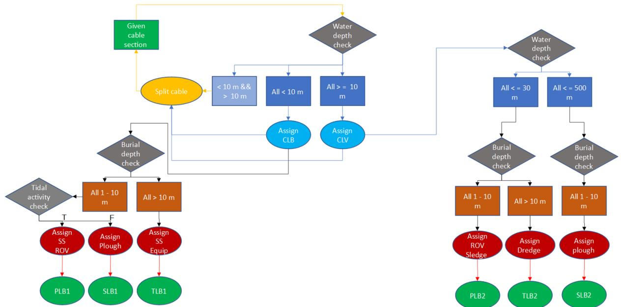
Figure 2.3: Decision tree representation for installation method choice in a MIP.
