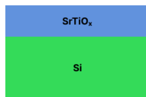
Figure 5.13: Thin film of strontium-titanium-oxide on a silicon substrate
