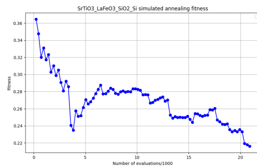
Figure 5.32: Multilayer stack of strontium-titanium-oxide, lanthanum-iron-oxide, silicon-oxide on a silicon substrate simulated annealing fitness
