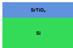
Figure 5.1: Thin film of strontium-titanium-oxide with Si substrate
