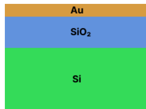
Figure 5.9: Gold film on a silicon-oxide layer on a silicon substrate
