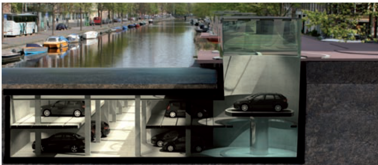
Figure 2: Impression of a parking garage underneath the Amsterdam city canals [De Ingenieur, 2007]
