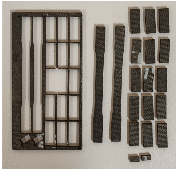
Figure B.4: Tensile and compression specimens of 30° before testing.
