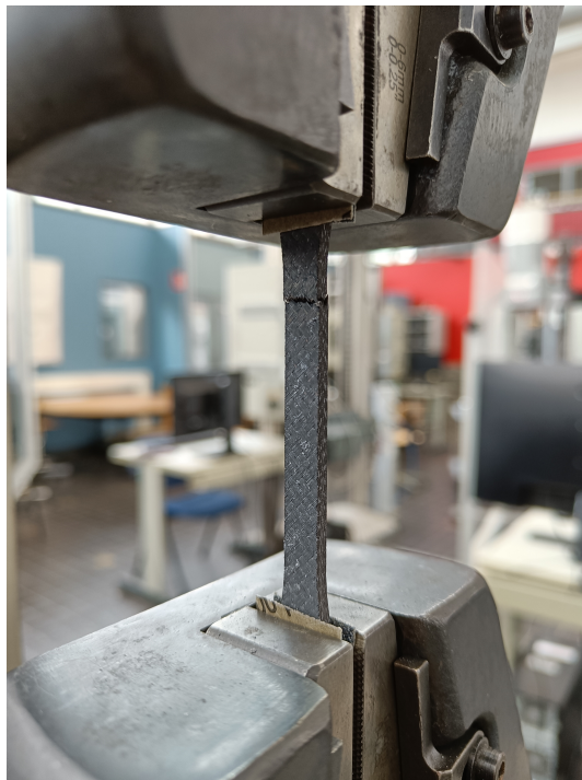
Figure C.3: Fractured tensile specimen after testing.
