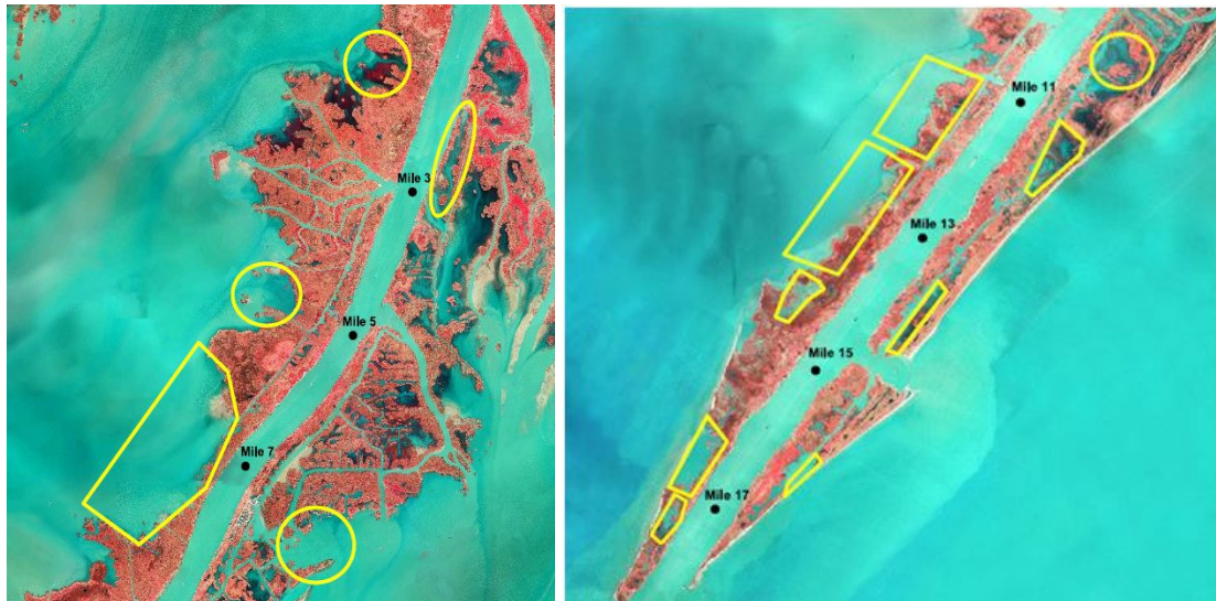
Figure C.1: Dredging strategy in the Southwest Pass at the mouth of the Mississippi River, from RM 0 to -17, Areas in yellow are Cutter dredger placement sites [USACE, 2010]
