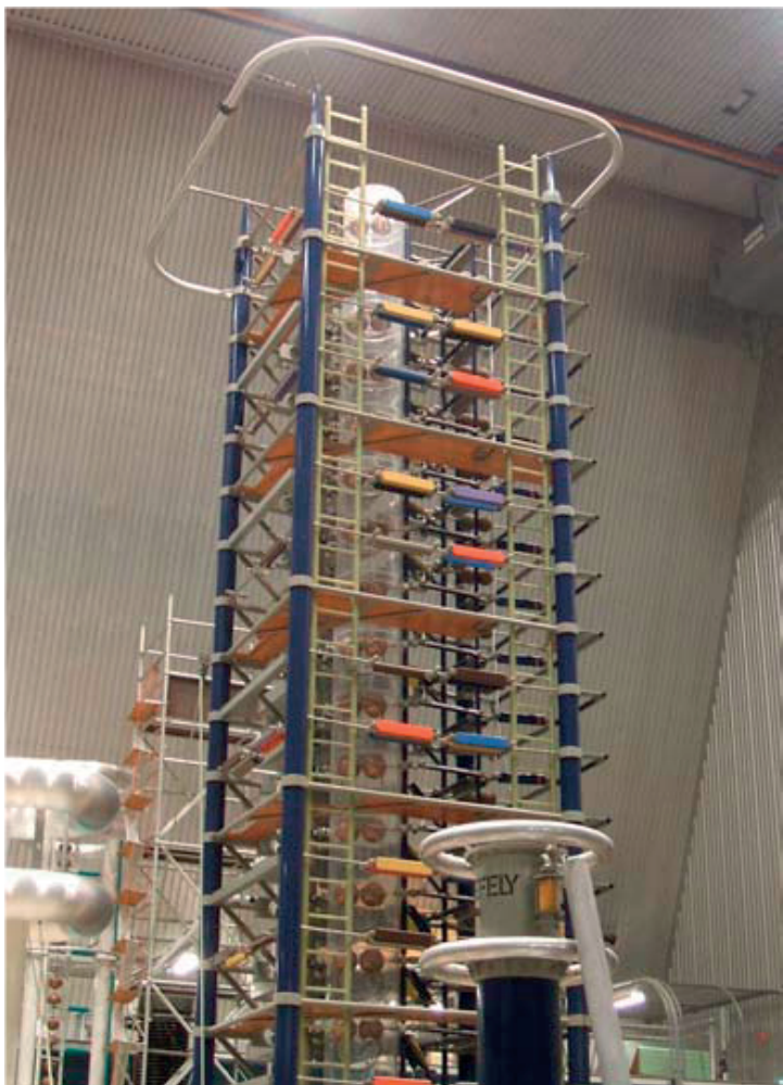
Figure 3.29: 20-stage Haefely impulse voltage generator.
