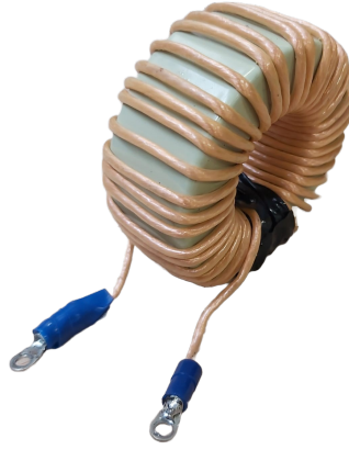
Figure 3.17: Lab-assembled inductor composed of a ferromagnetic core and a wire winded around it.
