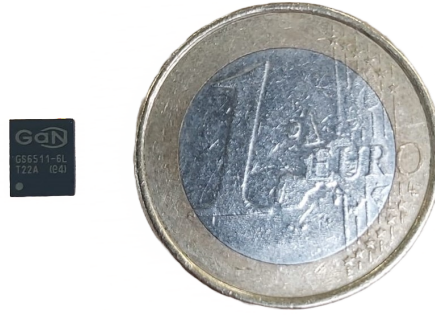
Figure 5.2: Size comparison between a GaN HEMT and a euro coin.
