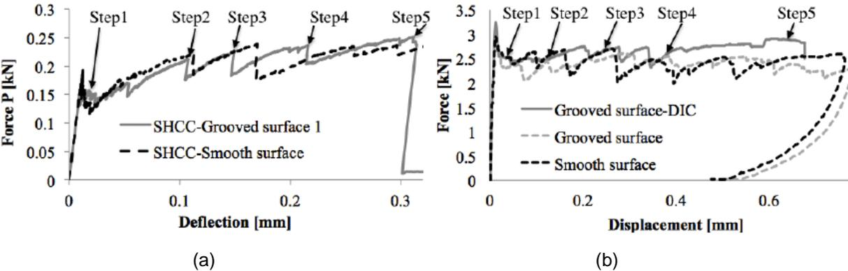
Figure 10: a) Simulated samples and b) Experimentally tested samples (Grooved surface – DIC I the specimen which was processed by DIC technique)
