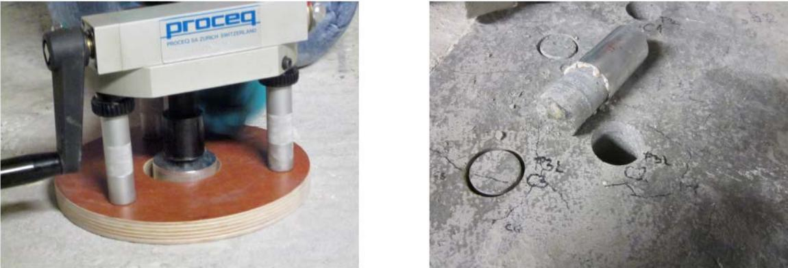
Figure 20: a) Pull- off test set-up and b) Typical failure mode in the substrate
