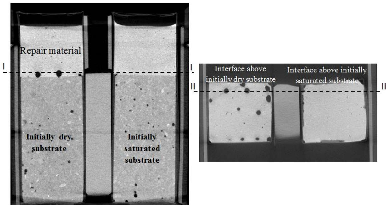
Figure 3: X-ray computed tomography images from repair systems with initially dry and saturated substrate made at the age of 3 days after casting the repair material with w/c of 0.3 (repair material thickness 15 mm, mortar substrate thickness 40 mm).
