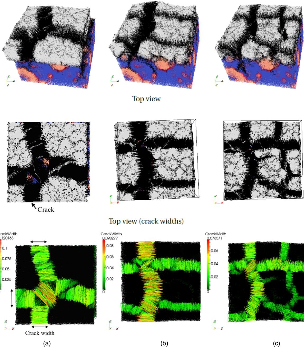
Figure 13 Resulting damage pattern due to restrained shrinkage deformation, influence of bond strength and substrate roughness on cracking after 110 days of drying in a) smooth surface, interface strength 1 MPa, b) rough surface, interface strength 1 MPa and c) rough surface, interface strength 3 MPa.
