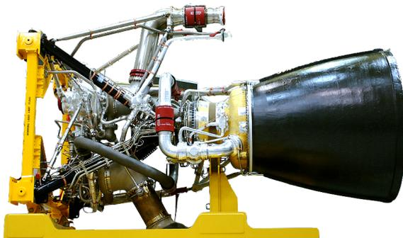
(a) Aerojet Rocketdyne RS-68 engine clearly showing a longitudinal load carrying structure consisting of four trusses<sup>1</sup>
