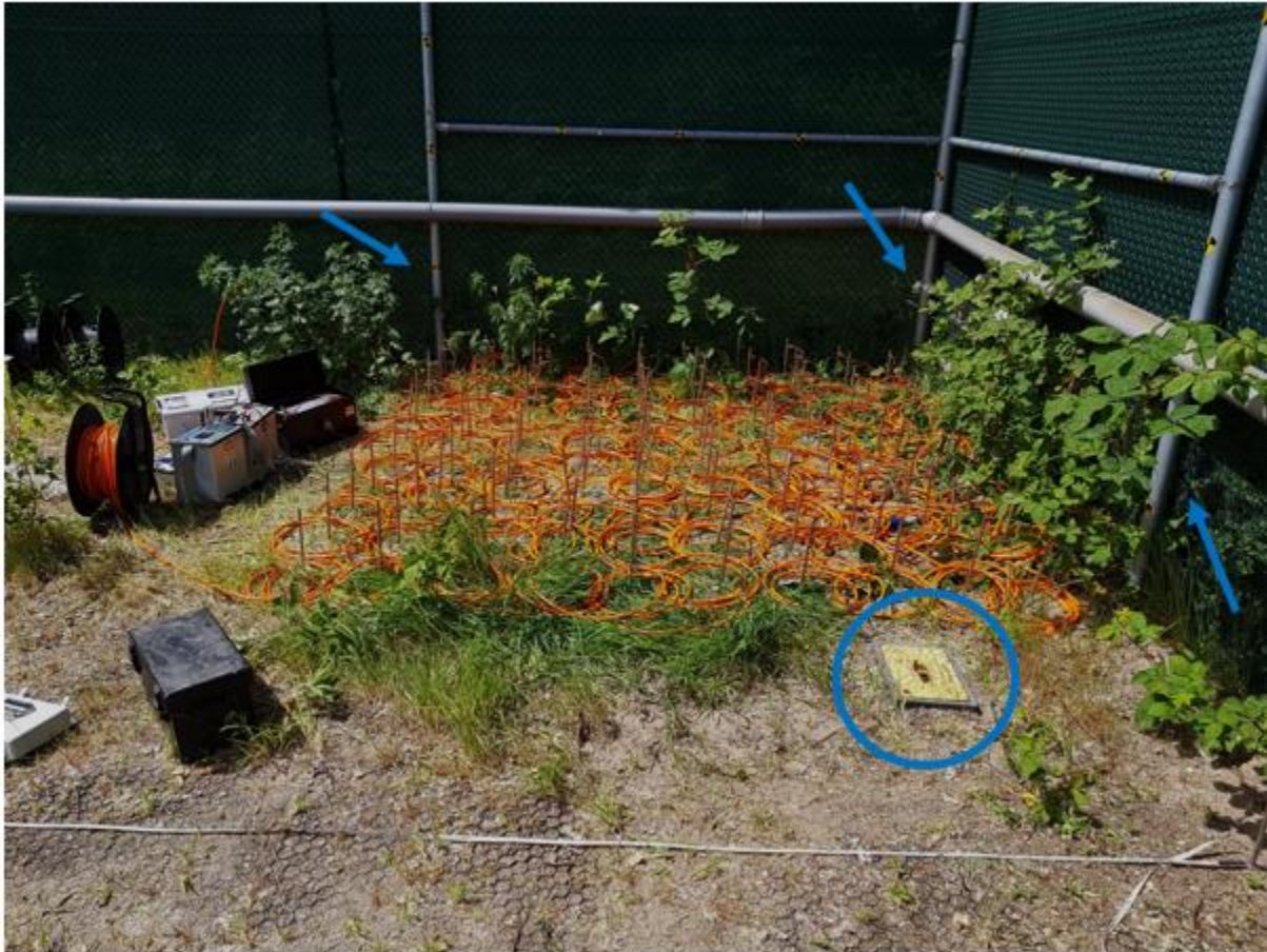
Figure 3.9: Photograph of resistivity survey setup at the ARISTA facility, with possible interferences marked by blue arrows and rings.
