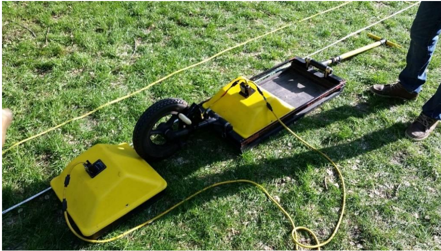
Figure 3.6: Photograph of multiple-offset GPR set-up before data collection.
