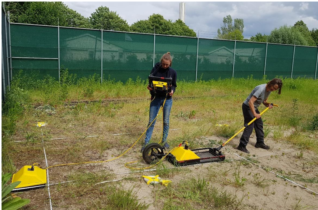
Figure 3.11: Photograph taken during the collection of a line of multiple-offset GPR data.
