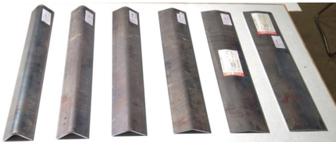
Fig. 2 4 mm thick specimens with different cold-formed angles
