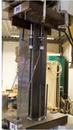
Fig. 3 Set-up for the compression tests
