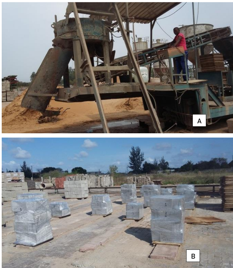
Figure 2: A: the equipment used to mix and mold the M15 concrete blocks. B: the blocks wrapped in plastic to keep the moisture.
