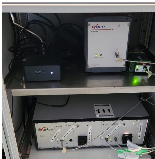
Figure 2.3: The two spectrometers inside the cabinet, featuring the UV-VIS and NIR spectrometers at the bottom and top respectively
