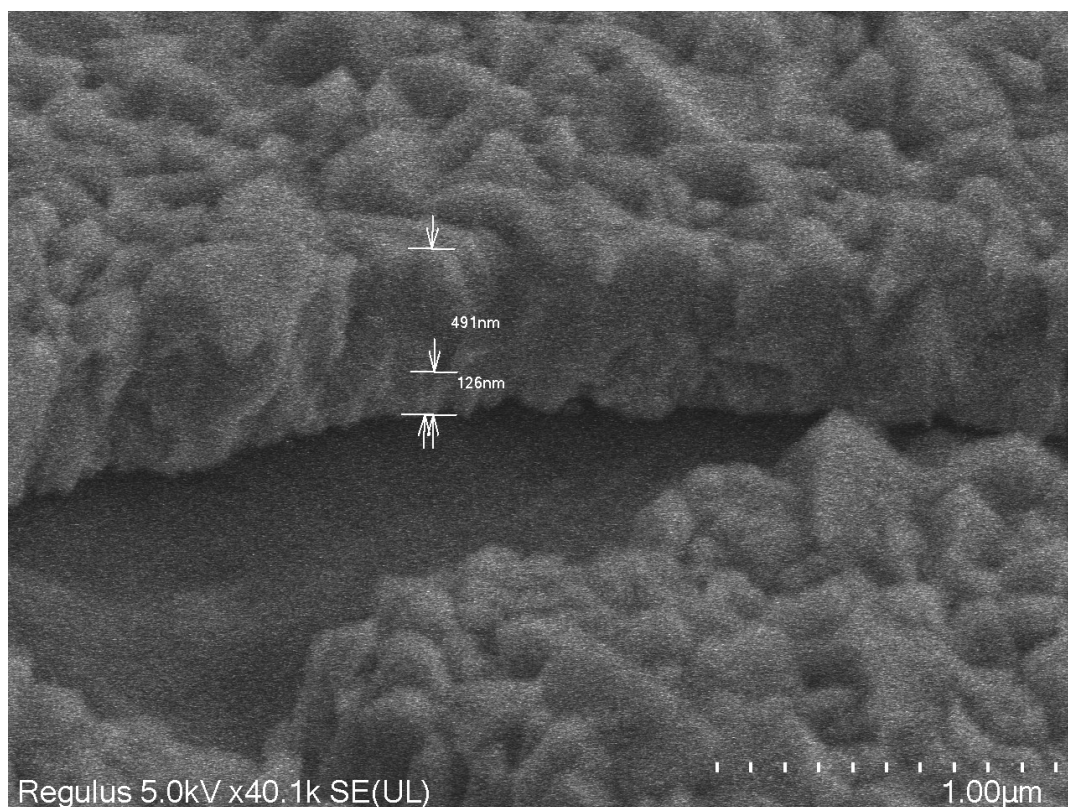
(a) A cross-SEM image taken at 1 micron resolution resulting in a total FTO thickness of 617 nm
