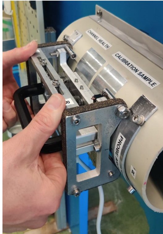
Figure 4.9: The WONDER device pressed against the channel health calibration sample to measure the voltage drops across each channel
